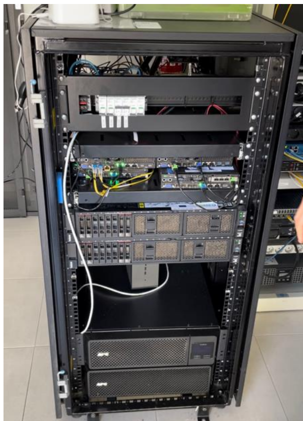
Figure 11: SR650 and SE350 Rack in the Control Room of the Cellnex Mobility Lab in Castellolí
